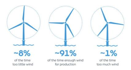
Figure 5. Average values of how often an offshore farm can produce renewable energy. Data based on North Sea wind farms (Ørsted, u.d.).
