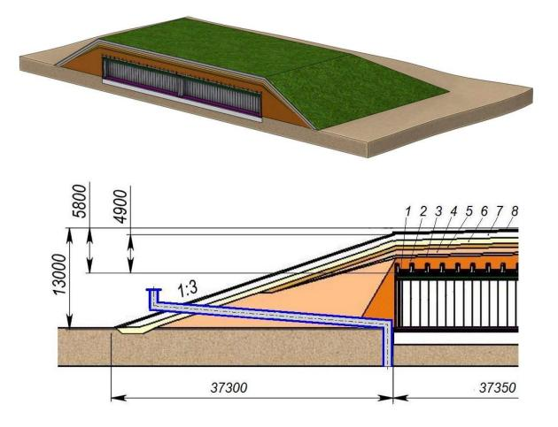
Figure S2. Image and composition (cross-section) of the 5.8 m thick engineered barrier after transformation of the storage facility (bld. 158) into the repository:
