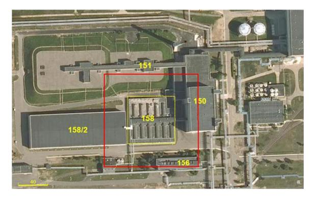
Figure S3. Reconstruction of bituminised radioactive waste storage facility (building 158) into the repository. The red line marks the 36 m wide area around the building, which will be used for the engineered barrier (multilayer cap)
