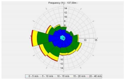
Figure 9. Wind rose for Kattegatt Syd, modelled for 137 m above the mean sea level.
