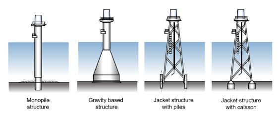
Figure 6. The different types of foundations currently applicable in Kattegatt Syd.
