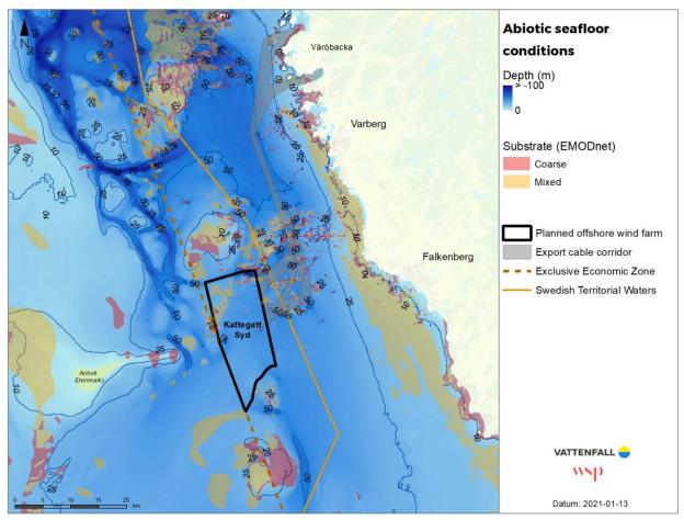
Figure 10. Depth and substrate conditions in the Kattegatt Syd area (data source: EMODnet).
