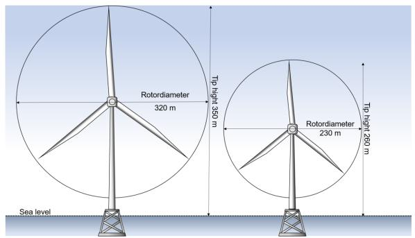
Figure 5. The relative size of the wind turbines for each wind farm layout example.
