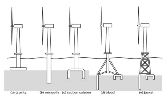
Figure 6 Foundations that typically constitute possible options for foundations for offshore wind turbines: a) gravity foundation, b) monopile, c) suction bucket foundation, d) tripod and e) framework (figur 3 i Oh et al., 2018).
