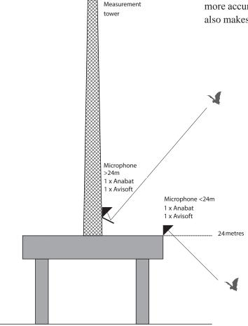
Figure 3. Outline diagram indicating the location of microphones on the measurement platform.
