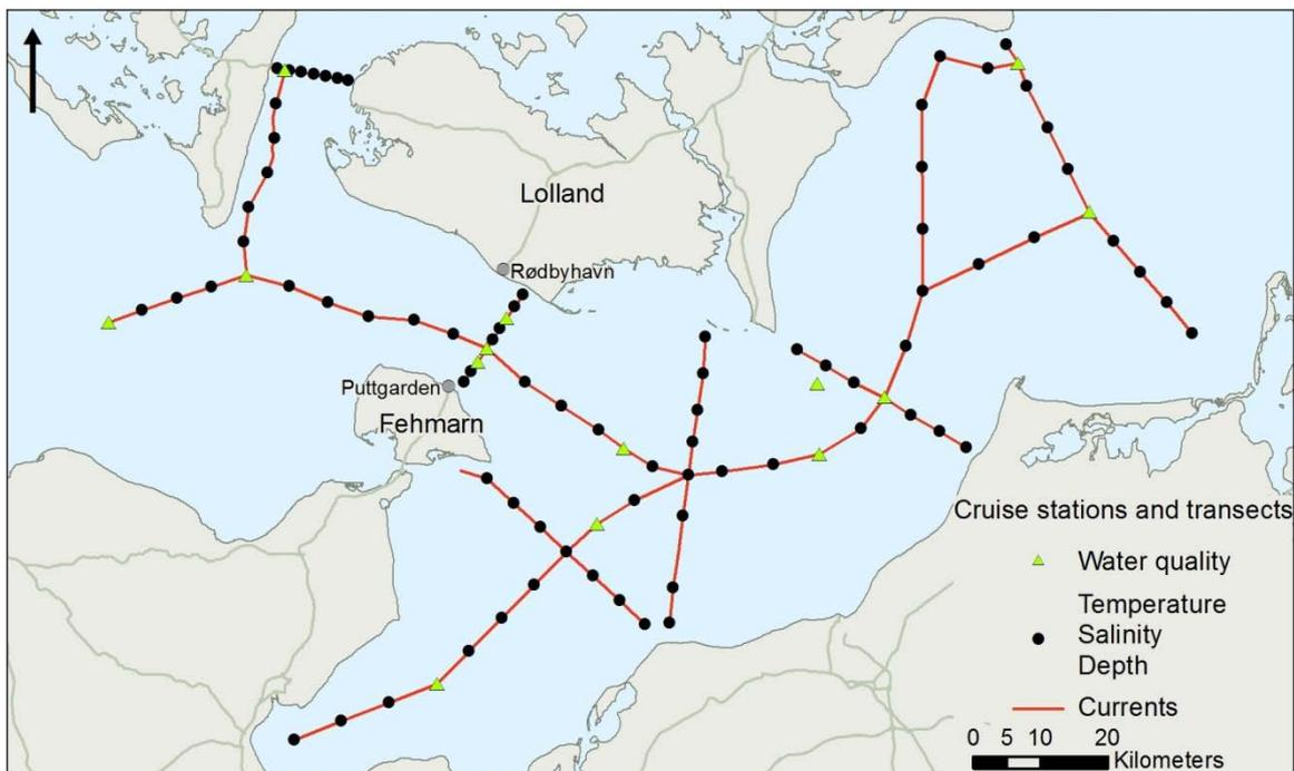
**Figure 7.3** The position of the 120 *in situ* monitoring stations and transects used to map hydrodynamic and water quality conditions.
