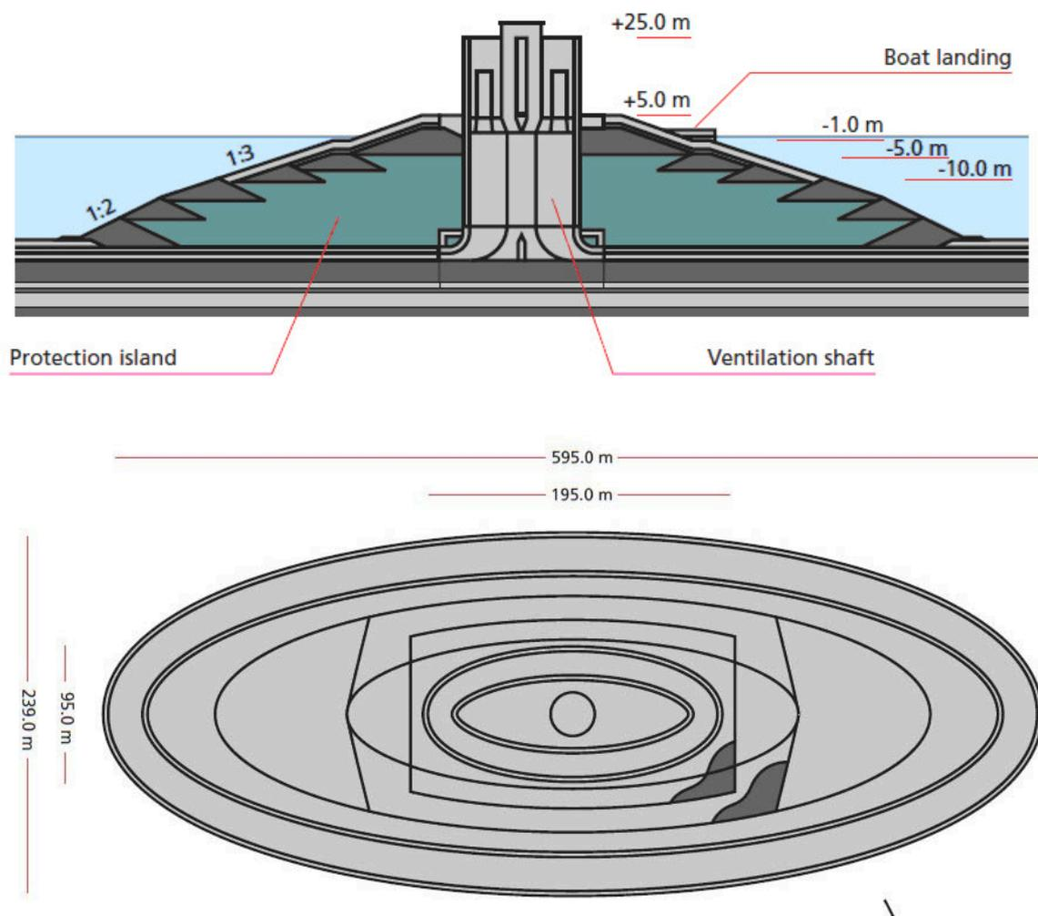
**Figure 2.6** Ventilation island of the immersed tunnel solution
