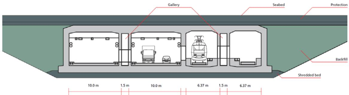
**Figure 2.5** Cross section of the suggested immersed tunnel solution
