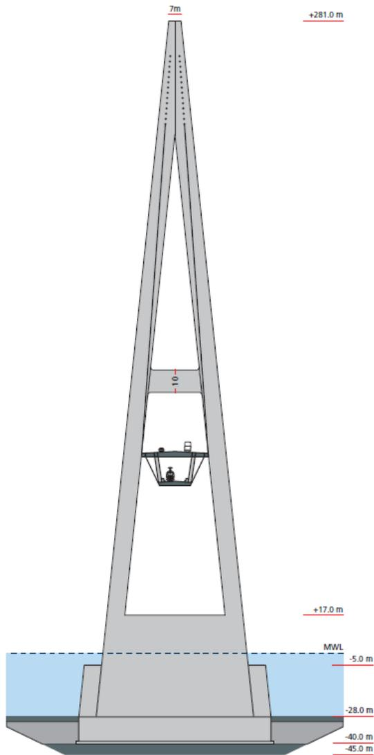
**Figure 2.4 Cable stayed bridge pylon**
