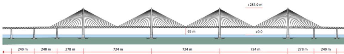
Figure 2.3 Lengthwise profile of the cable-stayed bridge solution
