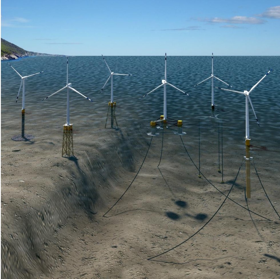
FIGURE 20 Overview of types of foundations for offshore wind turbines. Source: Illustration Joshua Bauer, NREL 49055.
