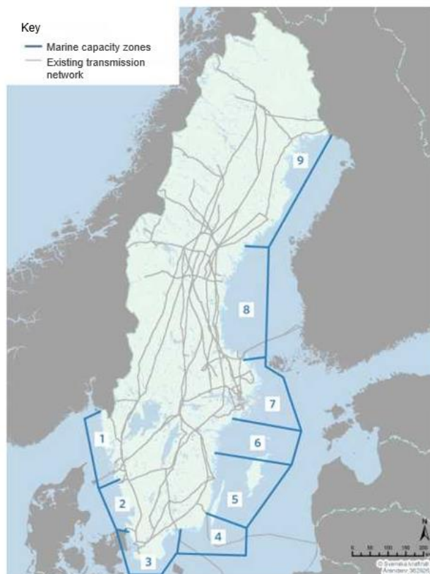
Figure 7.6-1 Svenska Kraftnät's marine capacity zones – grid capacity division of the Marine spatial plans. Skagerrak and Kattegat are divided into two zones (1 and 2), the Baltic Sea into five zones (3-7) and the Gulf of Bothnia into two zones (8 and 9). (SvK, 2022)
