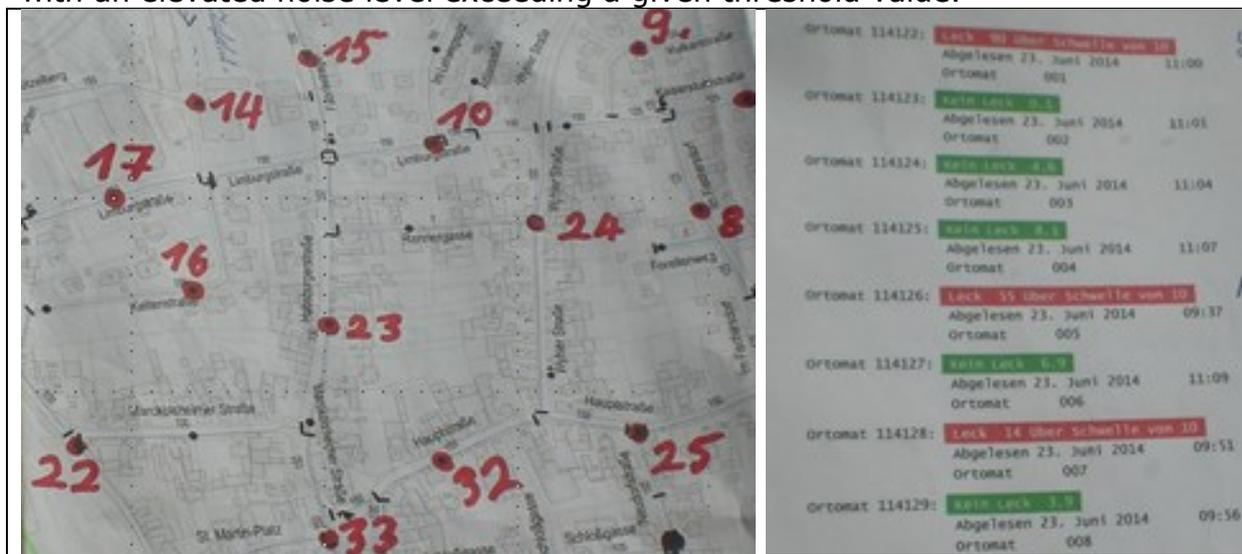
**Figure 10-13: Example of a part of a leakage monitoring zone where sensors/microphones with data logger (red numbers) have been positioned (left hand) and the automatic protocol indicating sensors/microphones with an elevated noise level exceeding a threshold value, marked in red (right hand)**
