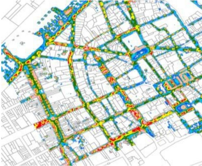
**Figure 3-11: Example of the final output of the analysis (after data processing to calculate illumination levels and its inclusion in a GIS system). Source: ALTILUM, 2013**
