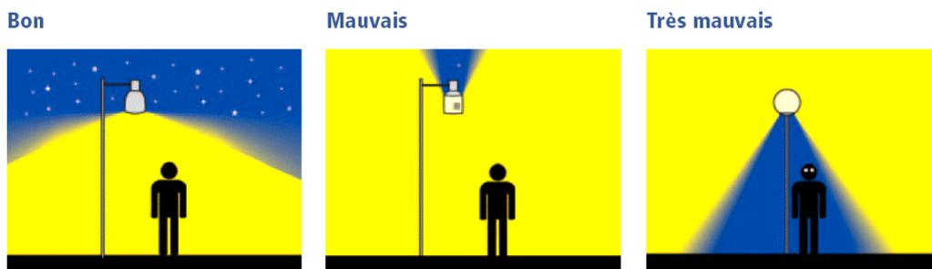
**Figure 3-9: Directionality of the lighting (Source: Bruxelles Environnement, 2011 – where the stated source is ASCN : <http://www.astrosurf.com/anpcn/> )**
