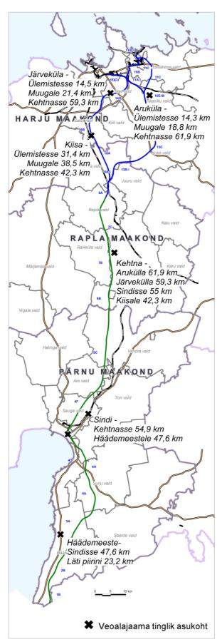
Principal locations of power substations/converter stations (marked with X) for Rail Baltic
