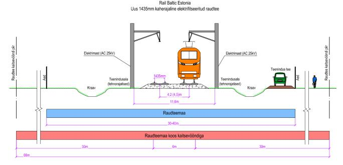
Cross-section of planned railway area in Rail Baltic corridor. The red line below marks the area necessary for planned railway and railway protection zone (66 metres), blue line stands for land needed for railway only (30-40 metres).
